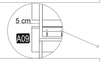
If the pre-drilled holes dont allign with the metal, dont worry please install the metal part as shown in the figure
