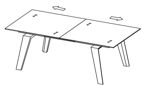
Tip: pull the side glass until the extension part pops up completely.
