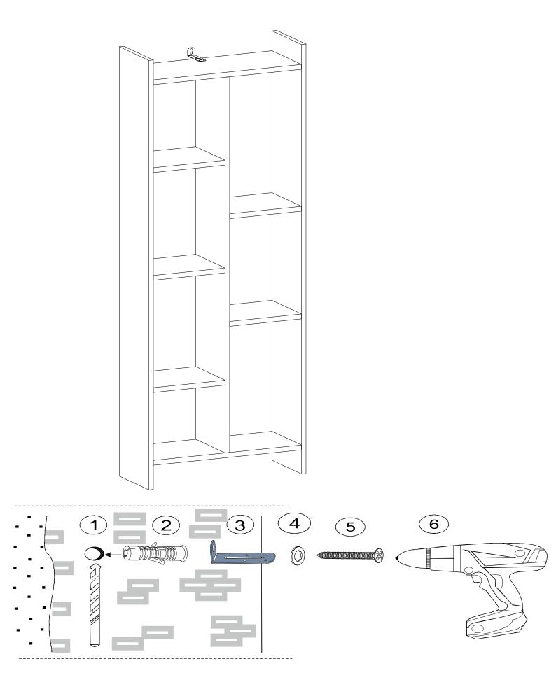
Check the Wall type before installation of dowel. Wall is drilled with equal diameter of dowel.(08mm) Universal Plastic Dowel provides the general purpose usage. Requires two stages assembly. Dowel can be different type according to the wall type. (e.g. Plaster Sheet Partition Wall, Gas Concrete, Hollow Brick Wall) If required, use appropriate dowels and screws.
